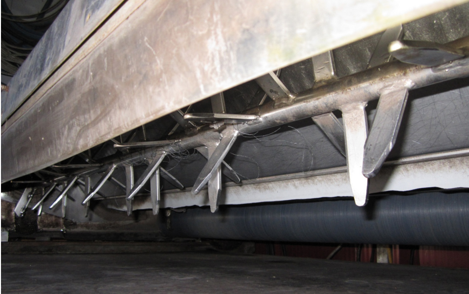
Figure 7.4 Detail of a ruffling machine: rod with teeth and pressure roller.
