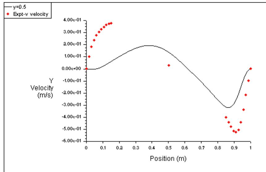
Figure 1.5: Calculated Vs. Experimental Data for Y-velocity on  $y=0.5$
