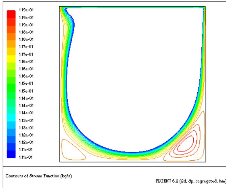
Figure 1.11: Contours of Stream Function with Vortices
