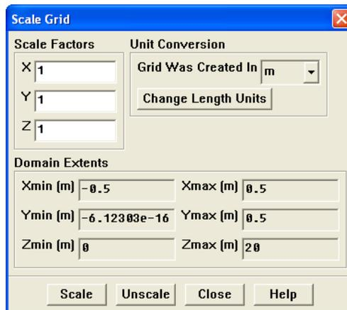
*Check the domain extents to see if they correspond to the actual physical dimensions. Otherwise the grid has to be scaled with proper units.*
