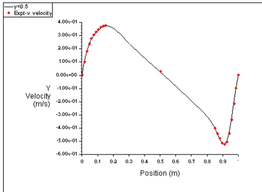
Figure 1.8: Calculated Vs. Experimental Data for Y-velocity with Higher Order Solution
