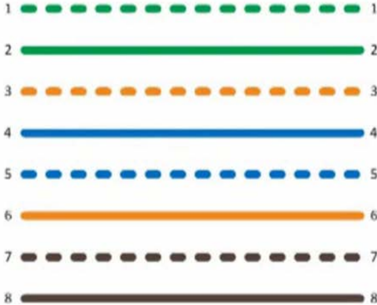
TIA/EIA 568A Straight Through Cable
