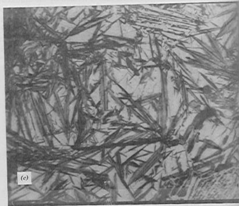
FIGURE 8-15 (b) Pearlite microstructure in 0.77% C steel, \times 1500 . (Courtesy of Dr. S. T. Jazwinski.) (c) Martensite microstructure in carbon steel, \times 1500 . (Courtesy of Dr. R. Jones, Lafayette College.)
